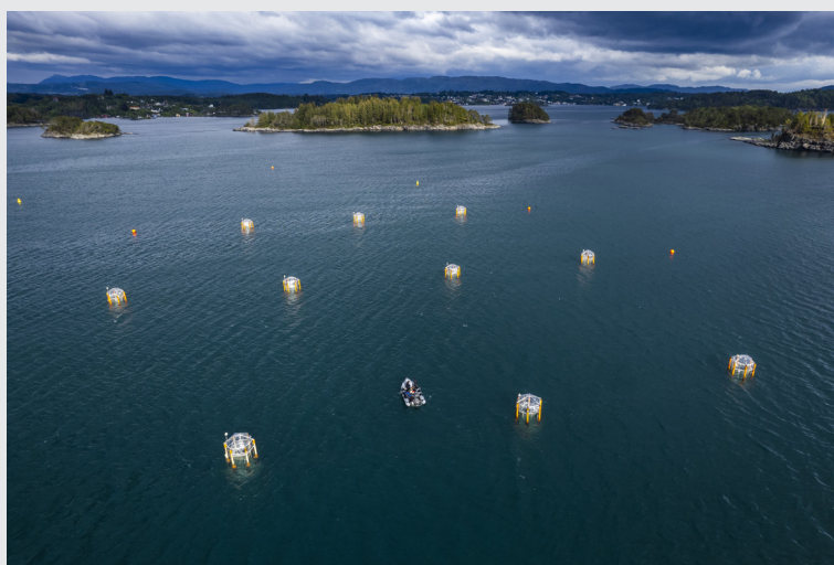
Figure 5. Mesocosm study on the effect of ocean alkalinity enhancement using the Kiel Off-Shore Mesocosms for Ocean Simulations (KOSMOS) conducted in the Raunefjord, Norway, in 2022. Photo by Uli Kunz.
