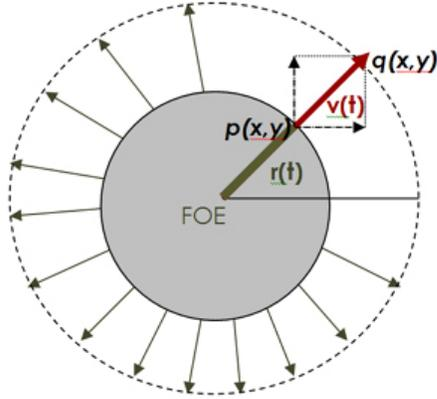
Fig. 7. Example showing the parameters for calculating the TTC with the camera approaching a sphere.
