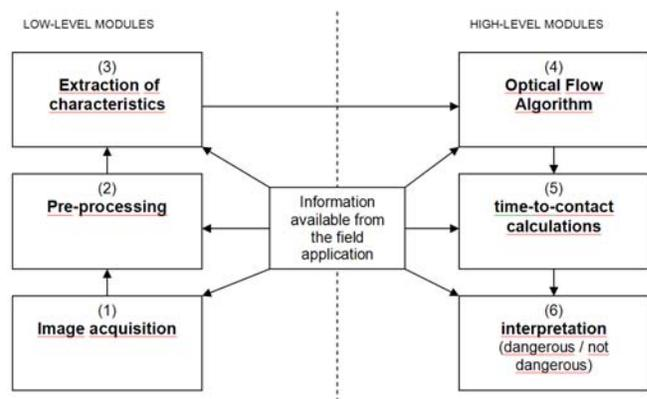
Fig. 1. Head-on collision detection system using artificial vision
