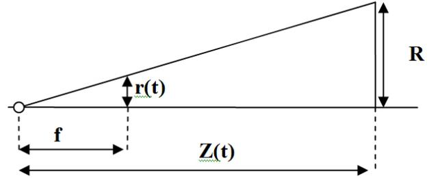
Fig. 6. Pinhole camera model.
