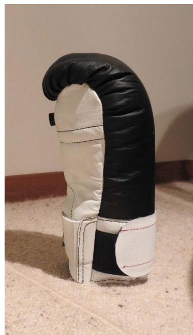
Figure 3. A prototype low-impact glove allowing air release and return. The port can be seen on the front surface of the glove toward the top.
