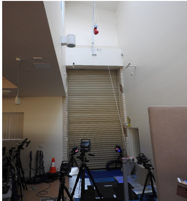
Figure 5. Drop testing system used for glove evaluation at the University of Canberra.
