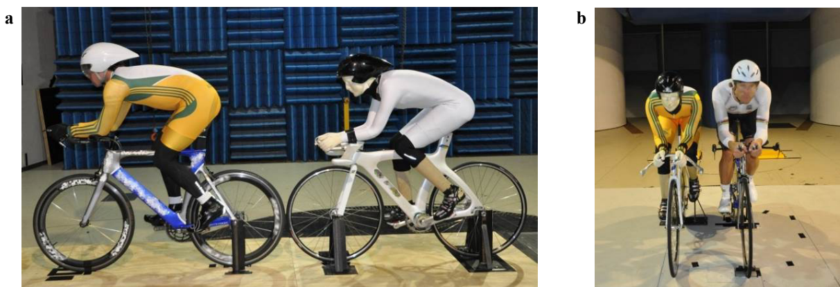
Fig. 1 (a) Drafting setup for trailing rider measurements— minimum separation shown; (b) Overtaking test setup at minimum separation
