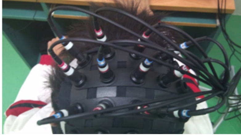
Figure 6.2: Optode positions used in the fNIRS experiments to prove activation and delay issue on a subject. There were three illuminators (blue) and three detectors (red) on each hemisphere. A pair of illuminator and detector optodes formed one channel on each hemisphere. There were totally 14 channels in the experiments.
