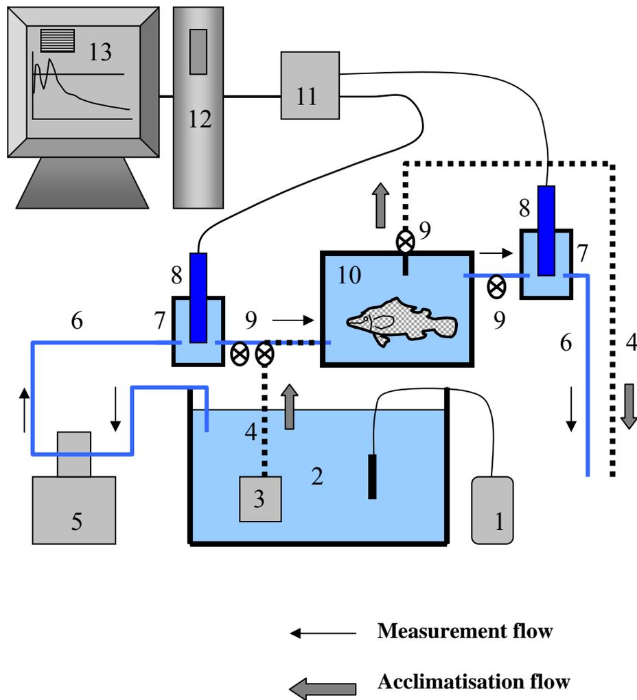
**Figure 2.4** Respirometer system consisted of (1) digital oxygen meter (2) water source, (3) submerged aquarium pump, (4) plastic tubes (5) peristaltic pump, (6) silicone tubes, (7) oxygen probe sockets, (8) oxygen probes (9) valve, (10) animal chamber, (11) oxygen meter and signal converter (12) data recorder in the computer CPU, and (13) computer monitor.
