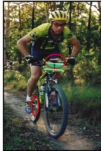
Figure 1. A MTB SRM power crank ([www.srm.de](http://www.srm.de)) and an SRM fitted to a cyclist's MTB.
