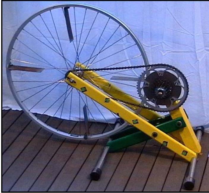
Figure 9. The Hayes Cycle Ergometer used for the Laboratory Simulation.
