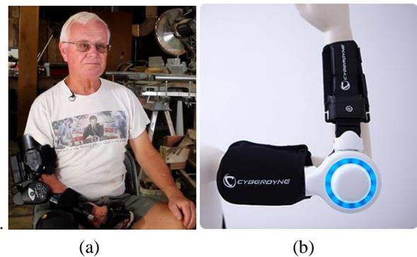
**FIGURE 6. (a) MyoPro exoskeleton for Veterans. (b) HAL for living support.**
