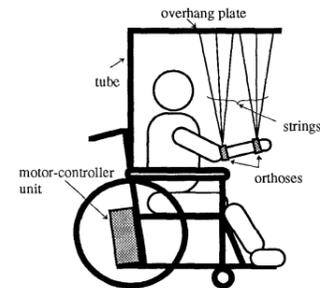
**FIGURE 4.** Upper limb assistive device concept.
