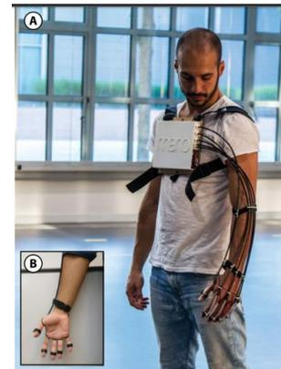
**FIGURE 10. Hand exoskeleton Mano.**
