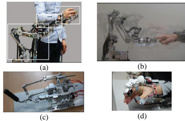
**FIGURE 9. (a) Overall system of 10-DoF upper limb exoskeleton KULEX. (b) forearm support part. (c) 3-DoF wrist part. (d) grasping part.**
