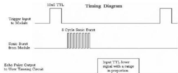
Fig. 6 - Timing diagram of ultrasonic sensor.
