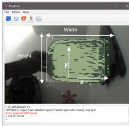
Fig. 3 - Signature setting using PixyMon software
