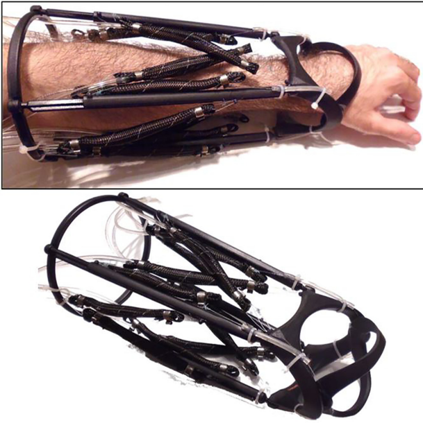
Figure 6: First prototype constructed for wrist rehabilitation robot using some redundant actuators.
