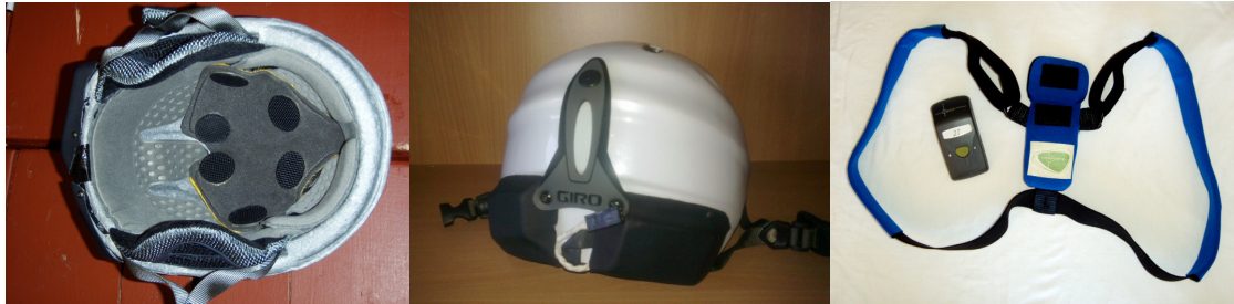
Fig. 1. (a) Giro-9 helmet fitted with accelerometers; (b) Giro-9 helmet showing placement of electronics; (c) GPSport SpiElite and harness
