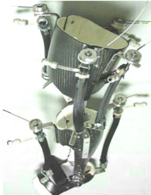
Figure 2–14. Knee–Ankle–Foot Robot from University of Michigan [95].
