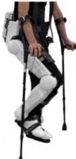
Figure 2–7. Hybrid Assistive Limb [82].
