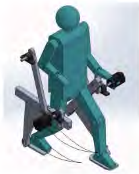
Figure 2-22. The proposed concept of the children's gait rehabilitation [96].
