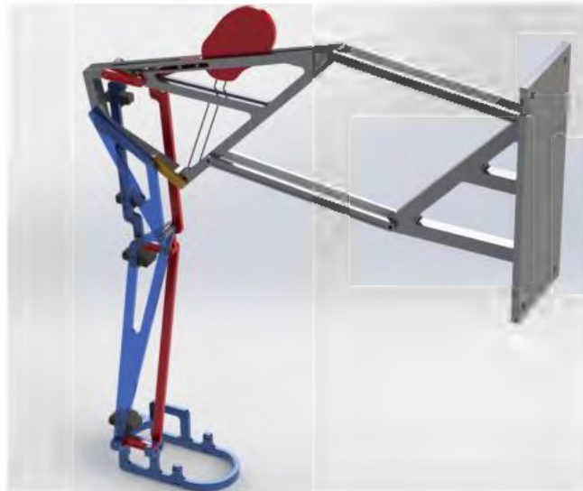
Figure 2-11. Six-bar linkage for ankle trajectory generation [81].
