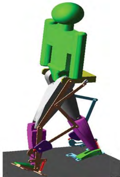
Figure 2-16. A simulation of the exoskeleton with a human subject in ADAMS software [88].
