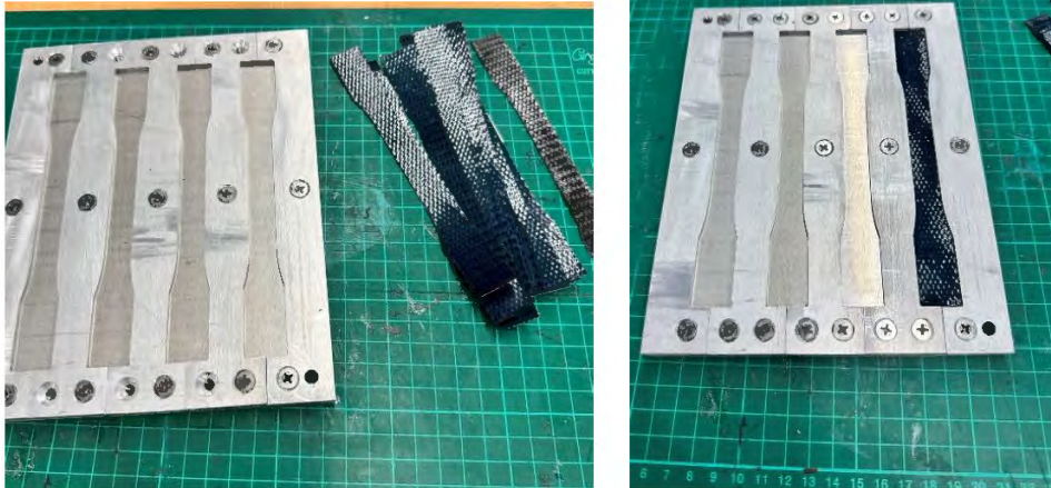
Figure 5.9 Stacking of prepreg layers to achieve the desired thickness.
