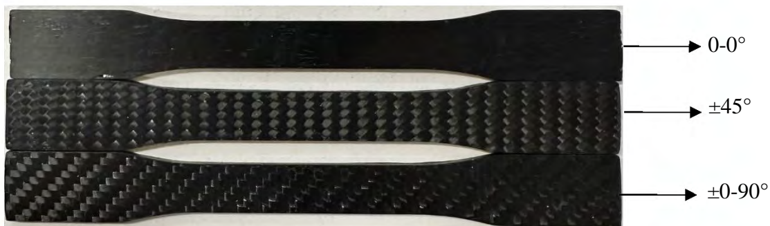
Figure 5.12 Tensile testing specimens at various fibre orientations.
