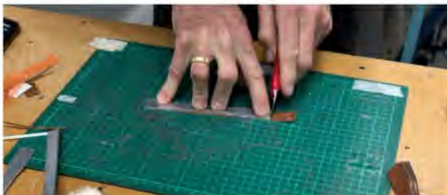
Figure 5.8 Cutting of carbon fibre prepreg to desired specimen shape.
