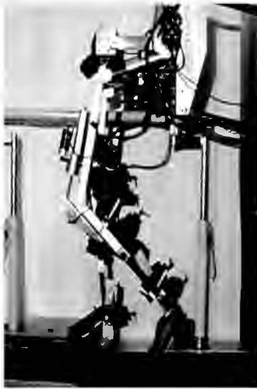
Figure 2.1 First clinical, steel prototype of the LOKOMAT system [50].
