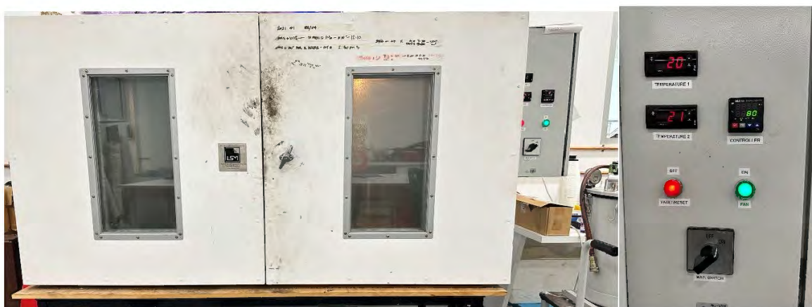
Figure 5.10 Air circulating oven to cure carbon fibre specimen.
